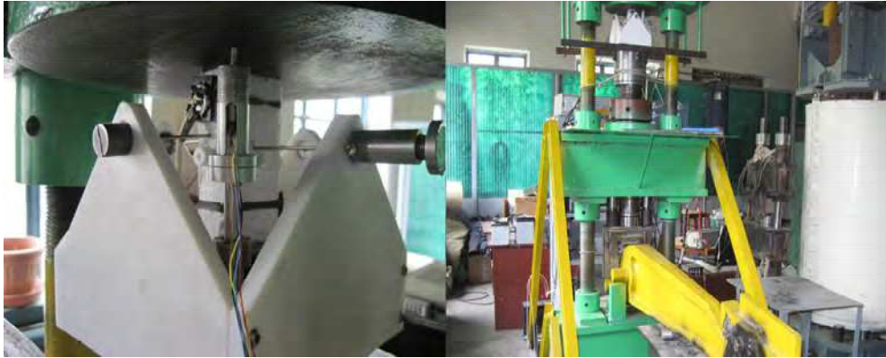
Fig. 1. Specimen with sensors and the lever press: a specimen with AE sensor, LVDT sensors of axial and lateral strain and electrode (the left frame); general view (the right frame)
