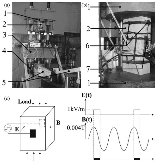
Fig. 1. (a) Lever machine UDI-L, (b) specimen installed for tests. (c) Scheme of experiment with Cr.EMF: at the left—the geometry: directions of main compression (vertical), electric field  $E$ , and magnetic inductance  $B$  are orthogonal, at the right—synchronization of periodical electrical pulses (G5-54) with AC generator supply to magnetic coil. Denoted elements: 1, loading platen; 2, specimen; 3, cross-arm; 4, supporting rod; 5, lever units clumping nut; 6, AE sensor; 7, electrode.
