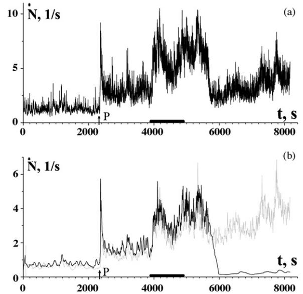
Fig. 2. (a) Temporal plot of AE activity, (b) the same plot with amplitude separation. Black bar on the time scale denote the influence of Cr.EMF; P–stress increment.
