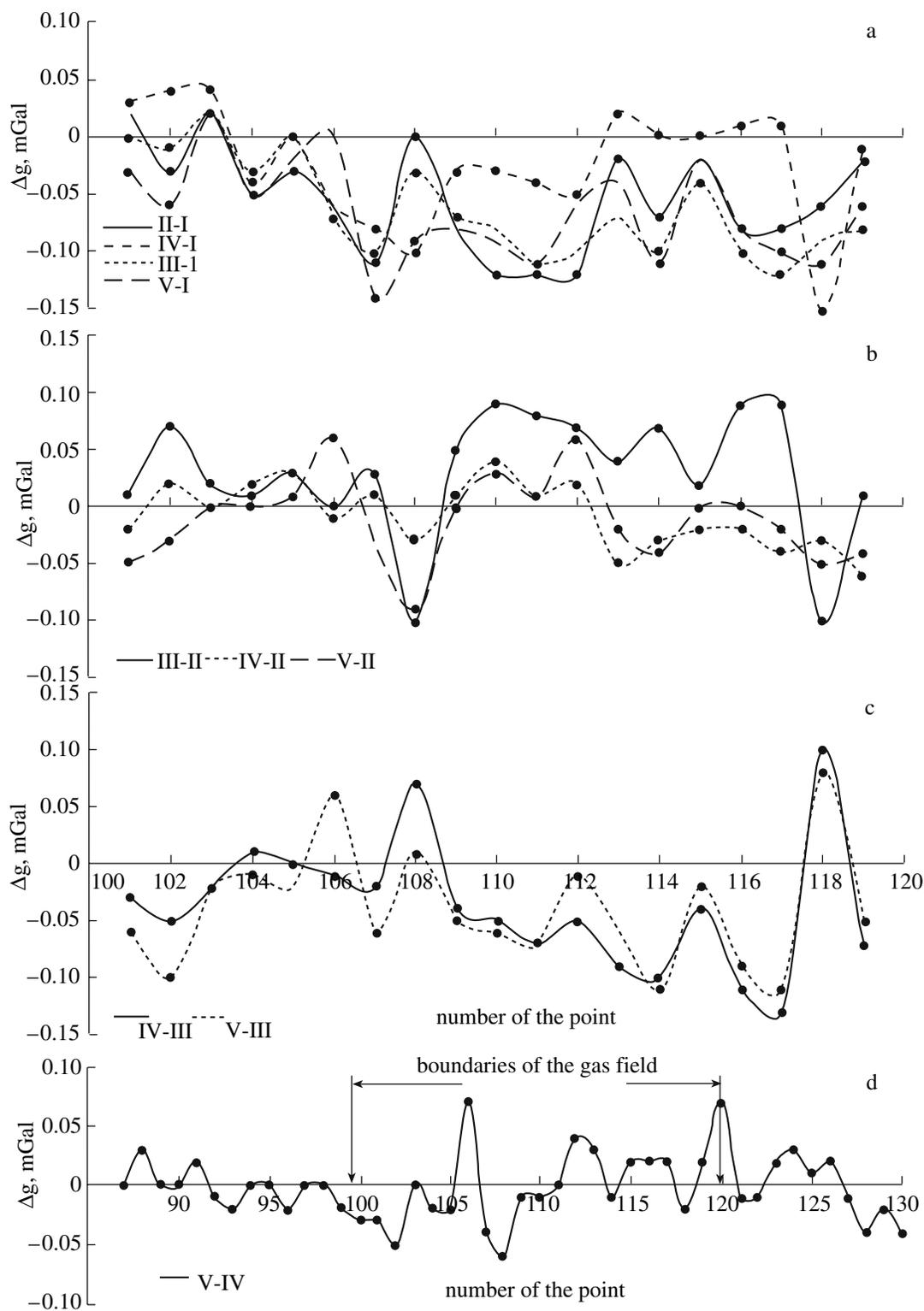
**Fig. 3.** Gravity differences between cycles of observations along profile 1: (a) with respect to cycle I; (b) with respect to cycle II; (c) with respect to cycle III; (d) with respect to cycle IV
