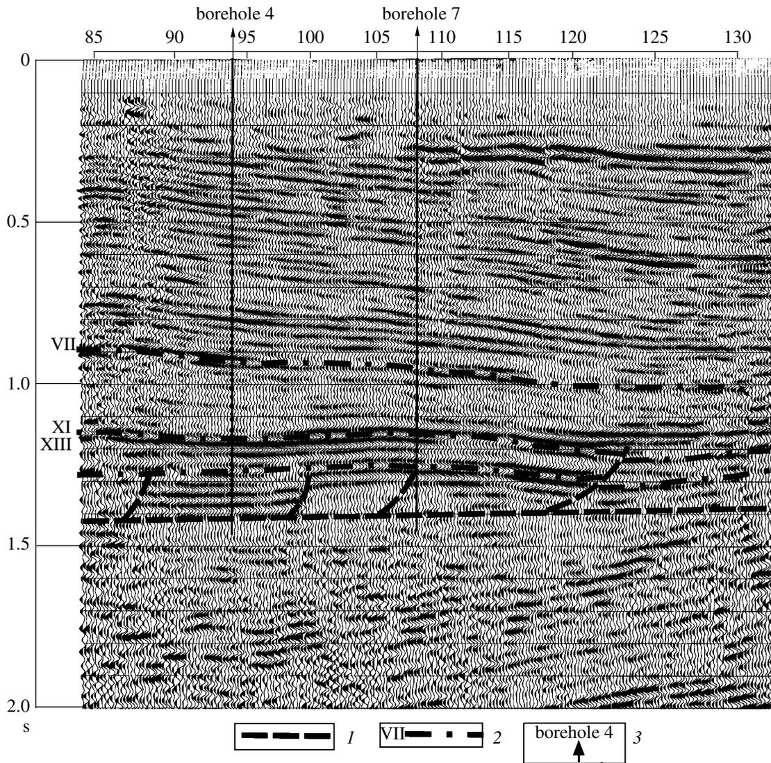
**Fig. 2.** Seismic time transect along profile 920205b in the interpretation of the authors (combined with profile 1 of the geophysical test site, see Fig. 1b). (1) Faults; (2) productive layers; (3) prospecting boreholes.
