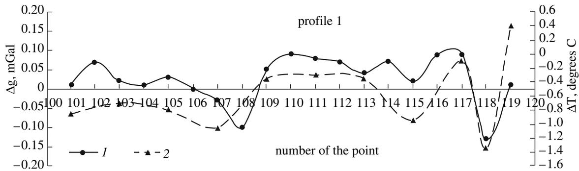
**Fig. 6.** Graphs of synchronous variation in the observed gravities and temperatures along profile 1 between cycles of observations III and II. (1) gravity differences; (2) temperature differences.
