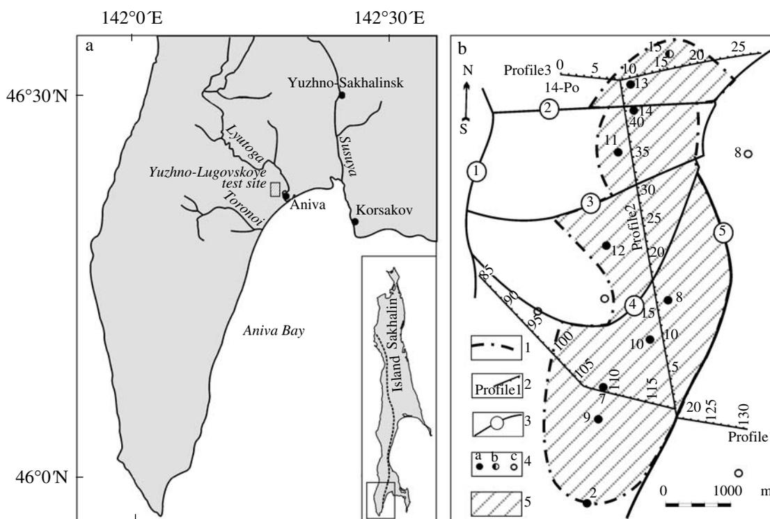
**Fig. 1.** Geographical location (a) and structural scheme (b) of the Yuzhno-Lugovskoye geodynamic test site in the southern part of Sakhalin (see the inset in Fig. 1a). (1) Boundary of the gas fields; (2) geophysical profiles; (3) main faults based on seismic and drilling data; (4) boreholes: (a) with economic influx, (b) with subeconomic influx, and (c) nonproductive; and (5) area of the gas field. The dashed line in the inset in Fig. 1a shows the location of the Central Sakhalin Fault.
