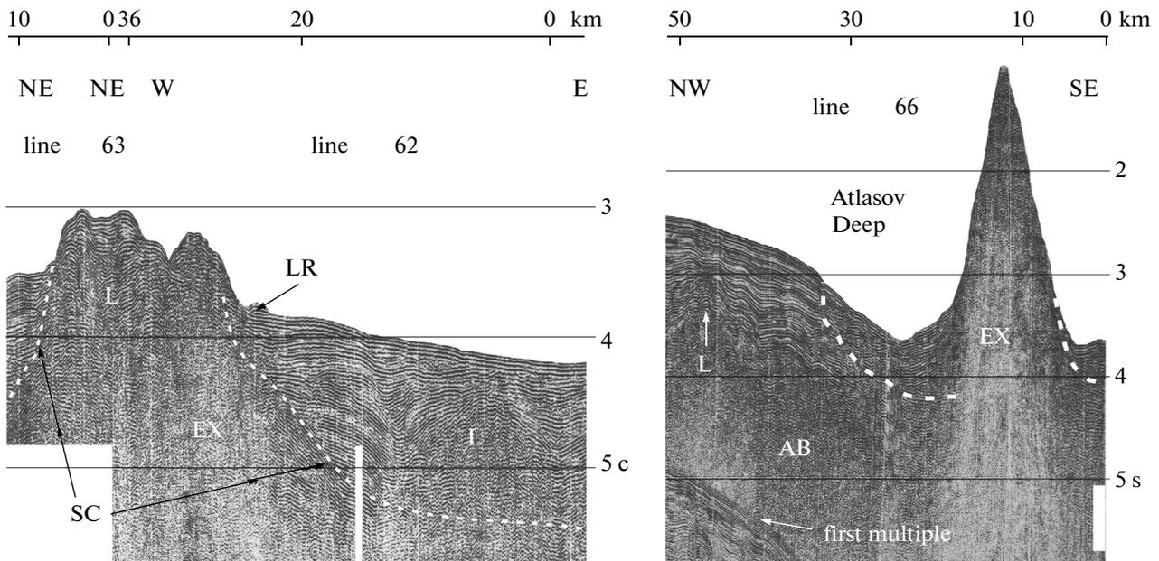
**Fig. 4.** CSP lines 62, 63, and 66, which illustrate the structure of laccoliths (L) or of subvolcanoes and of a cone of the two-summit extrusive mount in the Atlasov Deep.
