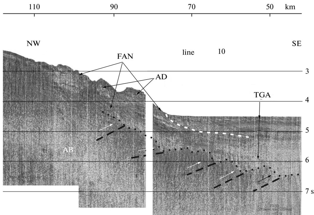
**Fig. 7.** A fragment of CSP line 10 across the accretion base with a fan of the canyon and the adjacent Sea of Okhotsk seafloor basin. AD aggradation dams that surround the fan valleys, TGA through-going anticline, dashed lines with arrows denote low-amplitude overthrusts of the acoustic basement (AB) and the direction of associated slip.
