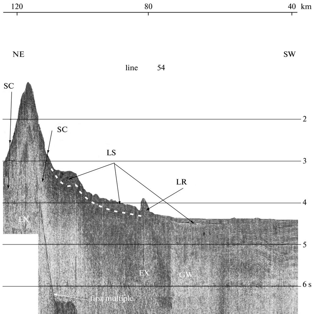
**Fig. 6.** A fragment of CSP line 54 across a block landslide at the base of an extrusive conical seamount and a flow landslide in the paleo-depression of the southern Sea of Okhotsk basin. For the notation see Figs. 2, 3, and 5.
