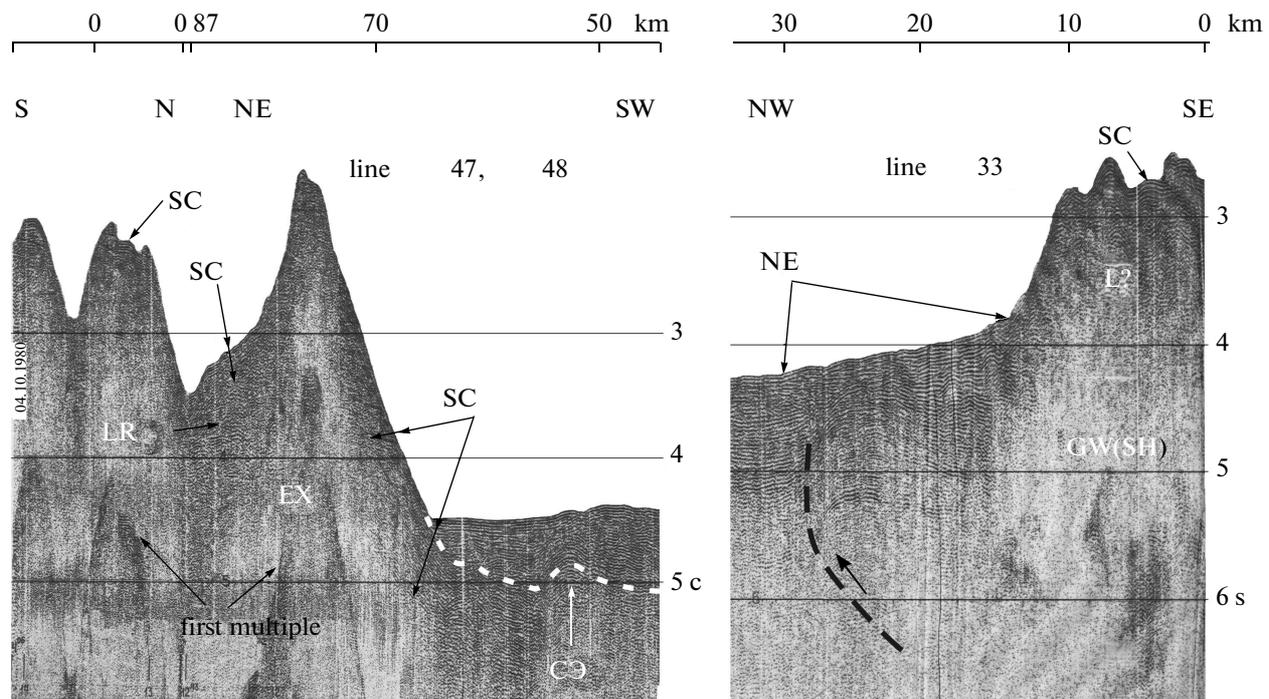
1 **Fig. 5.** CSP lines 47, 48, and 33 across the edge of an extrusive rock massif and a single laccolith. SC summit crater, BI blind intrusion, GW(SH) possibly a gas window or steam–gas hydrothermal occurrences, dashed line with an arrow beside it indicate a bottom overthrust and the direction of slip on it; for the other notations see Fig. 2.
