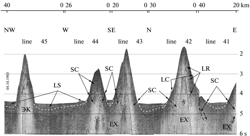
**Fig. 3.** CSP lines 41–45 illustrating the structure of a chain of extrusive conical seamounts. LC denotes lateral, probably extrusive, cones, LR stands for lateral reflections, LS denotes a small landslide at the base of the mount on the right of it and flow landslides; for the other notations see Fig. 2.
